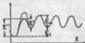
FIG. 3. One-dimensional model of the energy barriers to vacancy creation at a jog.
